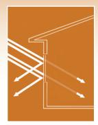
The "E" stands for "emissivity" but Low-E really means energy efficient. Low-E windows have a thin metal coating, virtually invisible from the inside, which allows light in but inhibits thermal heat gain. Low-E windows, like the Milgard SunCoat", add to energy efficiency in both the heating and cooling seasons — helping to prevent heat from coming inside during the summer and escaping during the winter. For more information about Milgard's Low-E products, visit www.milgard.com.
